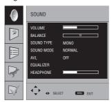
Balance: To adjust the sound balance between the right and left loudspeakers to the desired level, select the balance tab by using the downward direction (\*) button. Using the right/left direction (\*)/(\*) buttons, adjust the balance.
